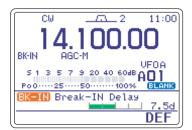
Delay time of 7.5 dots is selected for semi break-in operation.
